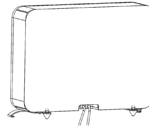
**C** Securely connect speaker wires (min 14 gauge AWG) through push-in binding posts. Be sure to preserve correct polarity with amp (red to red).
