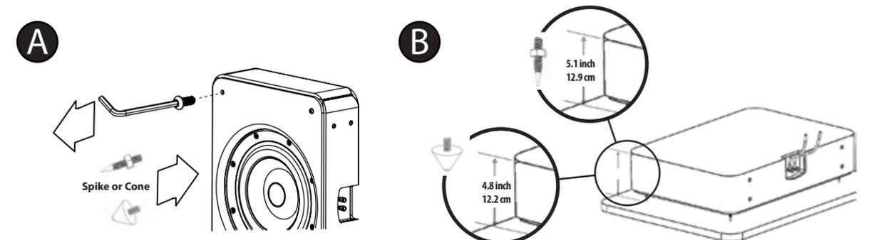
With grill off, remove all 4 button screws from enclosure face with Allen key; replace with included spikes or cone feet. Adjust so that all 4 feet make solid contact with floor or carpet without rocking or tipping. With spikes, remember to tighten the lock nuts.
