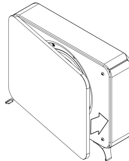
**B** Attach grill at one end; snap grill into place making sure that all 4 magnets are secure and that grill is snug all around.
