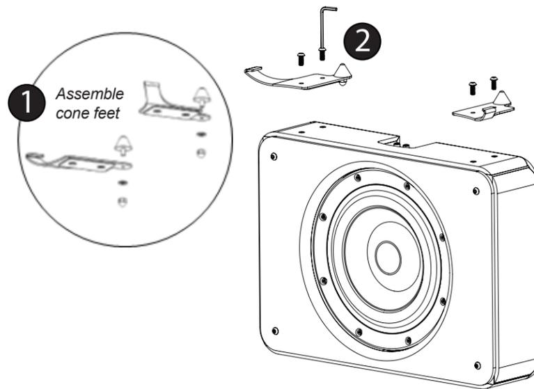
**A** 1: Attach cone feet to the standing feet with acorn nuts & washers (see insert). 2: With cone feet to the back of the enclosure, securely screw the 2 standing feet into the 4 inserts in the bottom of the enclosure with 4 button screws and 5/32" Allen key.
