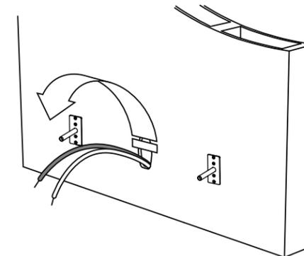
**C** Pull speaker wire through wire hole. Securely connect speaker wires (min 14 gauge AWG) through push-in binding posts. Be sure to preserve correct polarity with amp (red to red).
