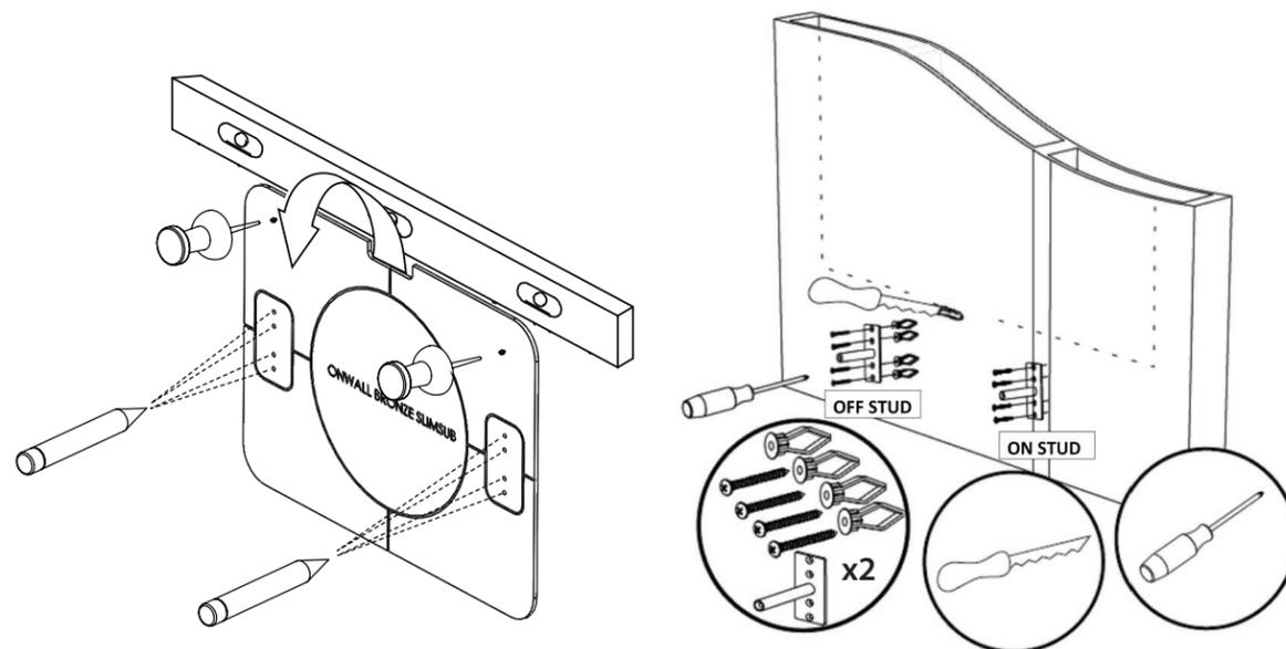
**A** Level & pin template to wall. Sub can be positioned horizontally (landscape) or vertically (portrait) with binding posts at either end. Outline wire hole and all 8 screw holes for 2 mounting posts. Screw post(s) into a stud if possible.
