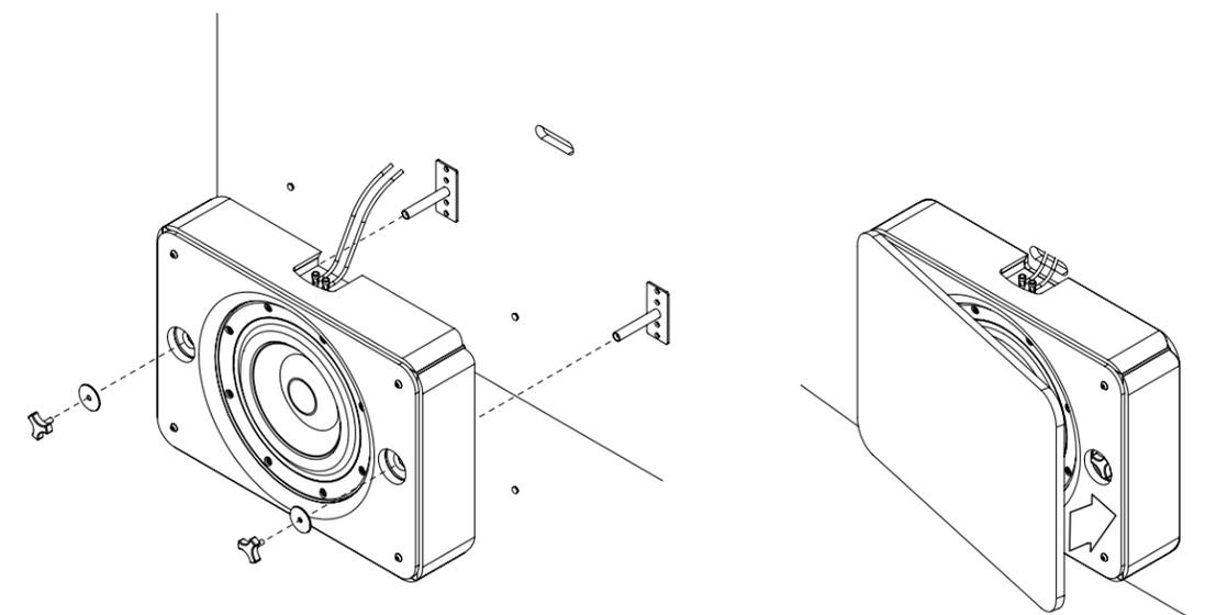
**D** Attach adhesive backed bumper to each of the 4 back corners. Mount speaker on posts; loosely tighten knobs through washers into posts. Level or align +/- 1/4" (6.35mm), then tighten both knobs.
