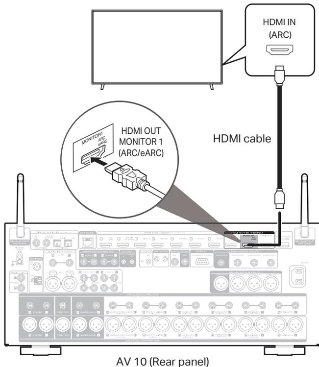
Using a high-quality HDMI cable\*, connect one end to the HDMI port labeled "eARC" or "ARC" on your TV. Connect the other end to the HDMI OUT MONITOR 1 port on your AV 10.
