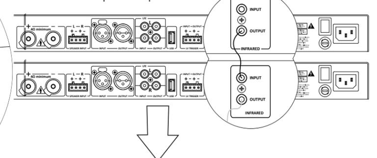
**Low Voltage Trigger** — Via snap in/pull-out phoenix connector. Input from low voltage (3-15V) trigger source. Daisy chain LV Output to next amp's input.
